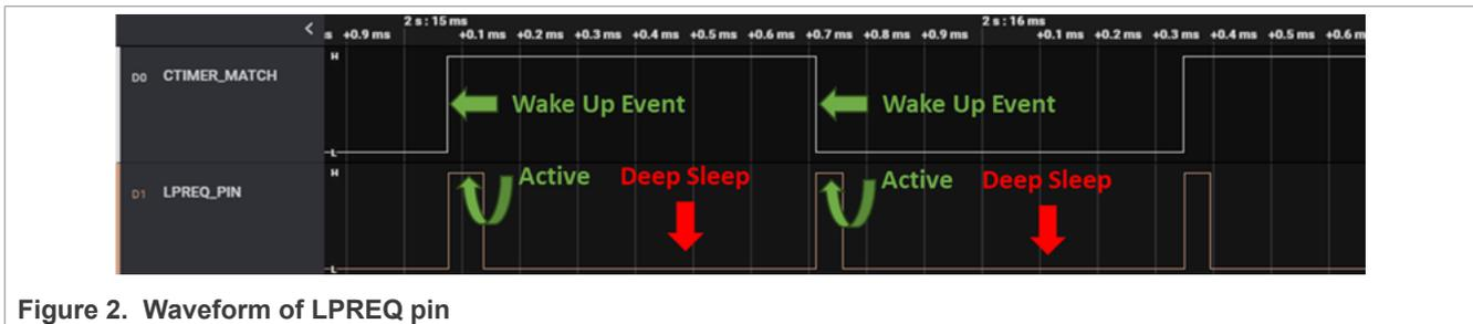
Figure 2. Waveform of LPREQ pin
